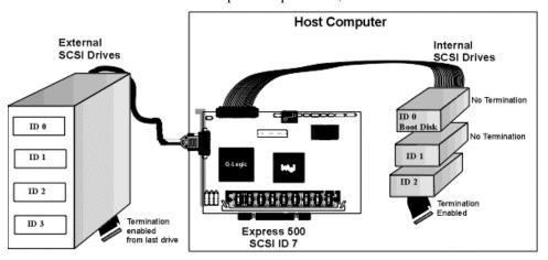
Connecting Non-Disk SCSI Devices SCSI Tape drives, scanners, CD-ROM drives, and other non-disk drive devices must each have a unique SCSI ID regardless of the SCSI channel they are attached to. The general rule for Unix systems is:
